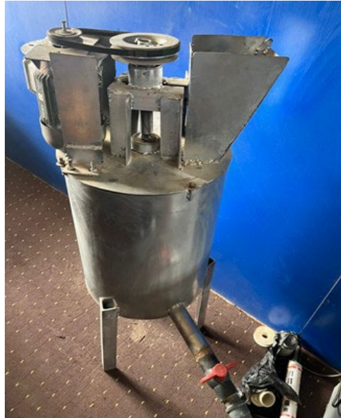
Fig. 13. Developed 50-litre batch capacity industrial mixer
